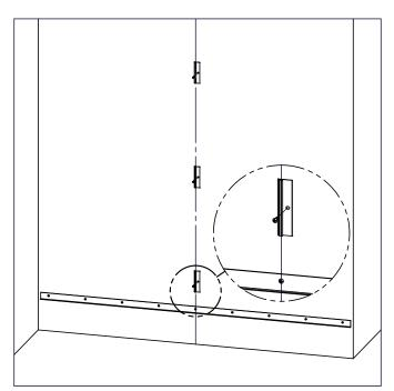
4) Using the vertical line as reference, install Intermediate Connectors as shown. Connectors should be installed 3-4" inches from each end of the AXIA profile and then spaced approximately 30-36" apart.
