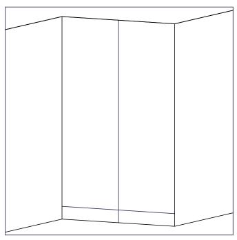
1) Draw a vertical line at the midpoint of the wall. If using an odd # of profiles, measure 2" to the left or right of the center line and begin there. Doing this will offset this first profile so each side is symetrical.
