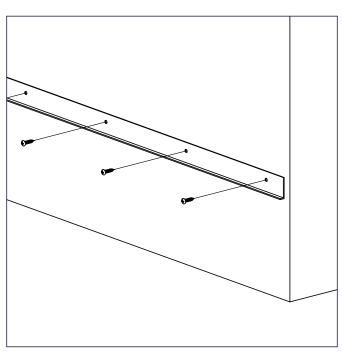
2) If the AXIA profiles will not rest directly on the floor or a baseboard, install an angle (or similar) to support the AXIA profiles.
