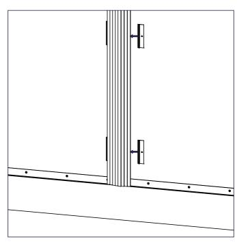
6) Secure the AXIA profile in place using Intermediate connectors. Make sure there is a tight fit between the connector and the profile before fastening the connector to the wall.
