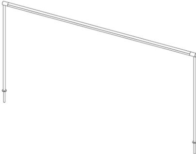
**General Description:** The Stylmark 11/16" diameter Showcase Reflector with Modular Light Engine is designed for commercial showcase displays that require a slim profile. Available in a variety of colors and finishes, the reflector can be mounted in wood end showcases using mounting hardware or in glass end showcases using down tube assemblies. Stylmark provides all hardware and electrical components for a finished assembly.
